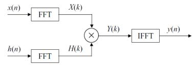
Fast convolution provides a significant reduction in computational requirements for higher order FIR filters, thus it is often used to implement FIR filtering in applications having a large number of data samples.
