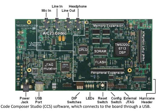
The DSK comes with a full complement of on-board devices that suit a wide variety of application environments. Key features include:
